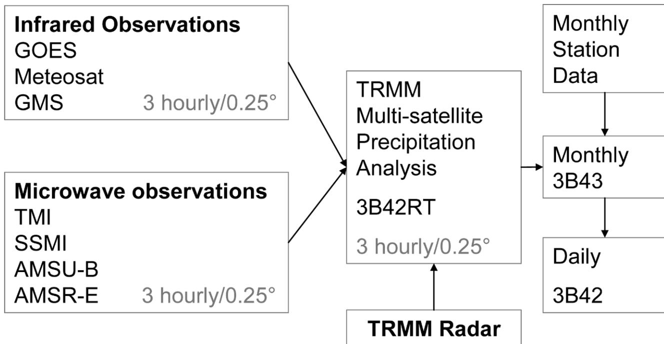
Figure 3: Schematic diagram of TRMM processing and outputs.
