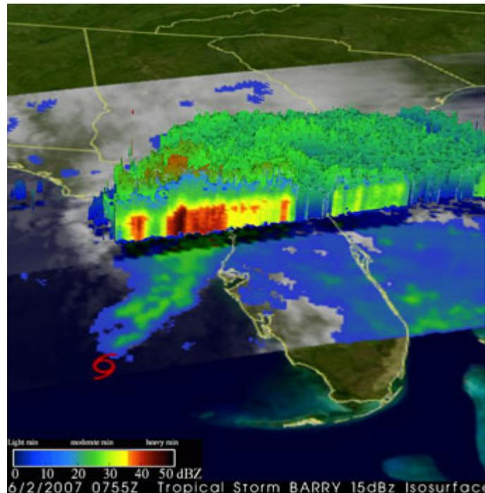
*Figure 2: The background image shows the horizontal pattern of rain intensities estimated from TRMM satellite data. Rain rates in the center swath are based on the TRMM Precipitation Radar (PR), and those in the outer swath on the TRMM Microwave Imager (TMI). The rain rates are overlaid on infrared (IR) data from the TRMM Visible Infrared Scanner (VIRS). [NASA image](#).*
